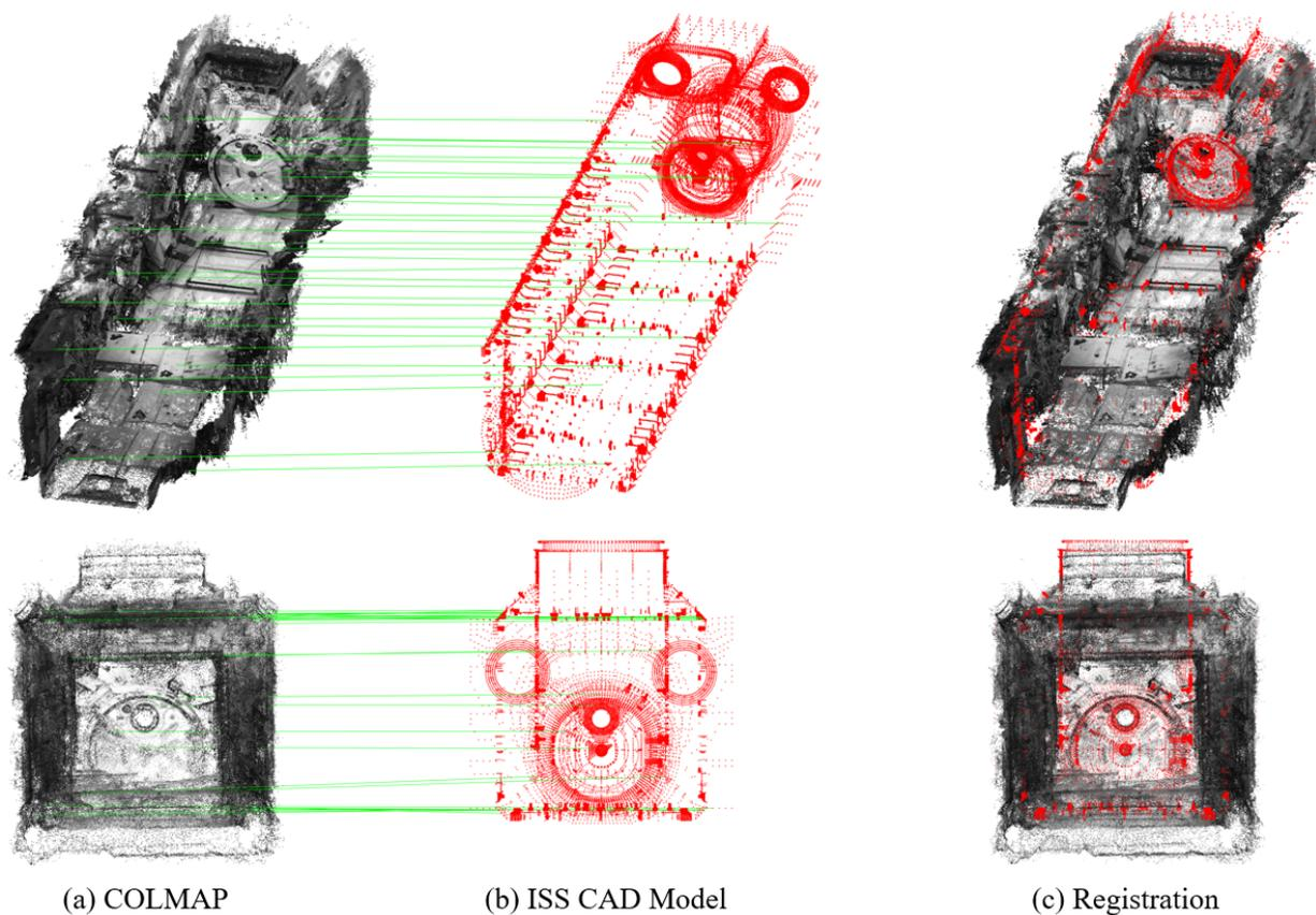
Fig. 4. Multi-view stereo (MVS) with the ISS CAD model. (a) Dense 3D reconstruction with COLMAP [1] given our pseudo ground truth 6-DoF camera poses. (b) Vertices (red) of the JEM 3D CAD model in ply format. We plot landmark pairs (green) between manually selected landmark points, showing consistent matching results. (c) The scale of the dense 3D point cloud from COLMAP is almost similar to the ISS CAD model (red), and they overlap consistently.
