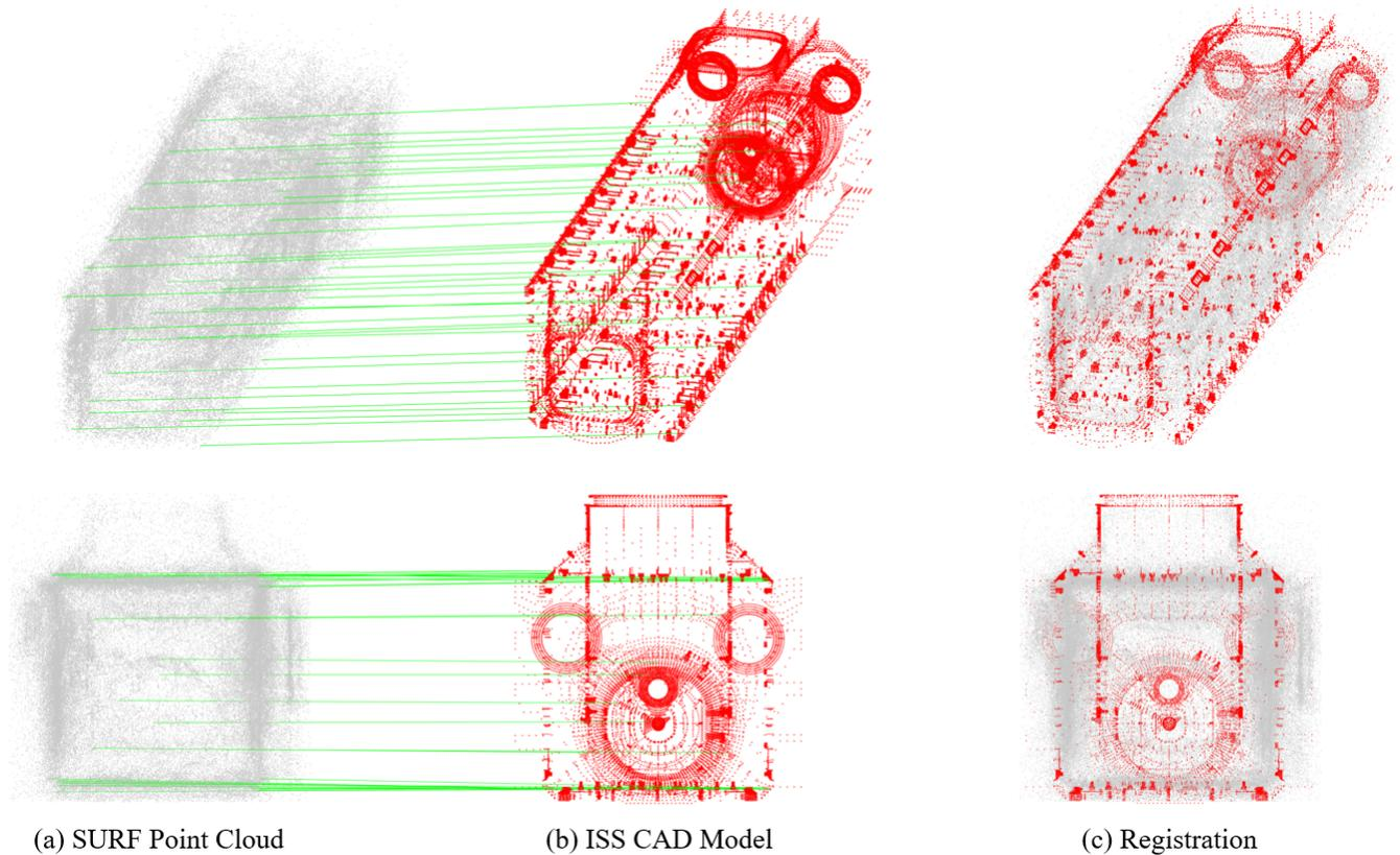
Fig. 3. ISS maps for ground truth generation with the ISS CAD model. (a) Our pre-built ISS maps consisting of SURF features (gray) used to generate the pseudo ground truth. (b) Vertices (red) of the Japanese Experiment Module (JEM) 3D CAD model in ply format. We plot landmark pairs (green) between manually selected landmark points, showing consistent matching results. (c) The scale of our pre-built maps (gray) is almost similar to the ISS CAD model (red).
