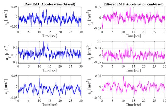
Fig. 1. Raw (blue/biased) and filtered (magenta/unbiased) IMU acceleration measurements obtained in the zero-g environment, i.e., on the ISS. We cannot find gravitational acceleration in the IMU acceleration measurements.
